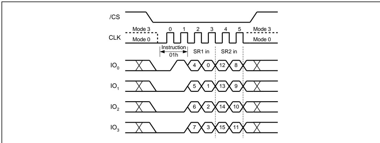
Figure 9d. Write Status Register-1/2 Instruction (QPI Mode)
