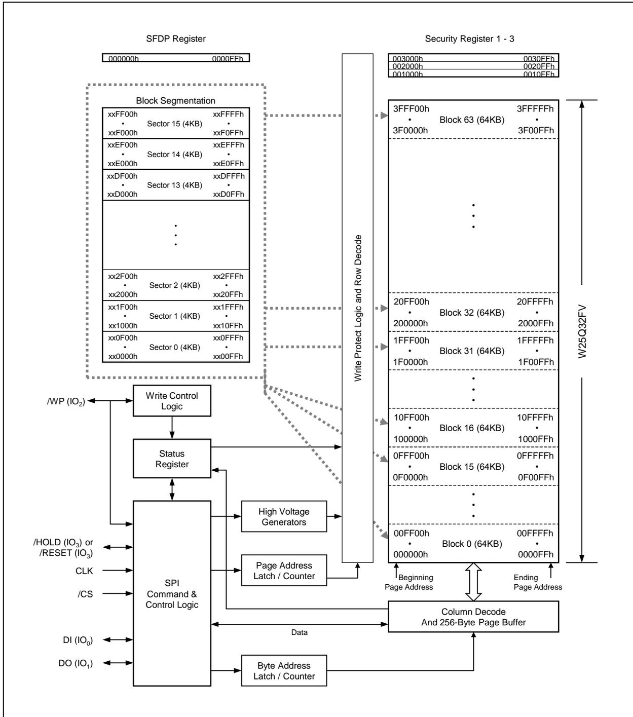
Figure 2. W25Q32FV Serial Flash Memory Block Diagram
