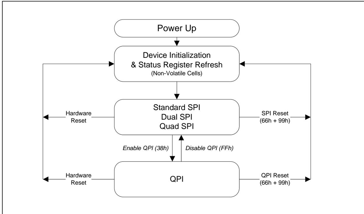
Figure 3. W25Q32FV Serial Flash Memory Operation Diagram
