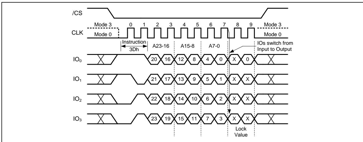
Figure 54b. Read Block Lock Instruction (QPI Mode)
